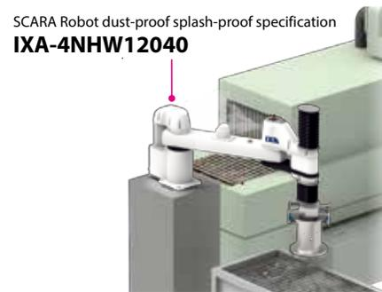
The IXA's dust-proof and splash-proof specifications are IP65 compliant, so it is not affected by water vapor. The IXA-4NHW12040 can handle a max. payload of 47 kg.
