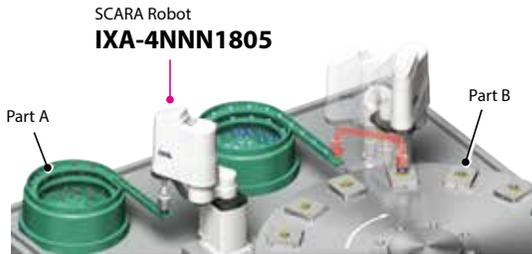
IXA, the fastest in the industry, also supports push-motion operation. When fitting part A to part B, the position error can be compensated (compliance control).
