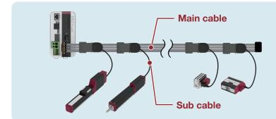
Run the main cable on the equipment and branch off the sub cables using dedicated connectors.
